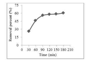
**Figure 4** Removal percent of direct blue dye by the selected acid activated durian peel (ADP-4) as a function of contact time at 150 ppm of initial concentration, pH 8 and 0.10 g/ 25 mL of dosage
