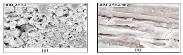
**Figure 6** Scanning electron micrographs of the selected acid activated durian peel (ADP-4) (a) before sorption (b) after sorption of direct blue dye
