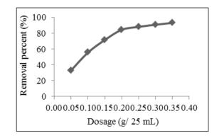
**Figure 5** Removal percent of direct blue dye by the selected acid activated durian peel (ADP-4) as a function of dosage at 150 ppm of initial concentration, pH 8 and 90 min of contact time
