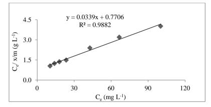
Figure 8 Langmuir isotherm: Sorption of direct blue dye by the selected acid activated durian peel (ADP-4)
