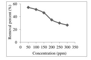
**Figure 2** Removal percent of direct blue dye by the selected acid activated durian peel (ADP-4) as a function of initial concentration at pH 8.4, 0.10 g/ 25 mL of dosage and 60 min of contact time
