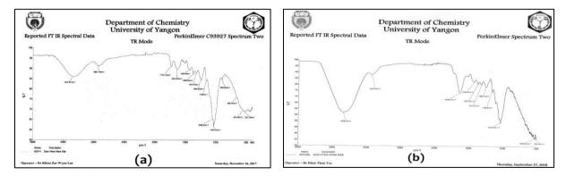
Figure 7 FT IR spectra of the selected acid activated durian peel (ADP-4) (a) before sorption (b) after sorption of direct blue dye
