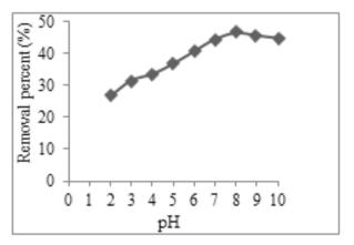
**Figure 3** Removal percent of direct blue dye by the selected acid activated durian peel (ADP-4) as a function of pH at 150 ppm of initial concentration, 0.10 g/ 25 mL of dosage and 60 min of contact time
